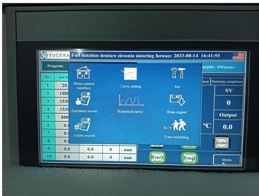
Main menu — Main control interface / Curve setting / Set / Operation record / Historical curve / Data export / Alarm record / Exit / User switching
